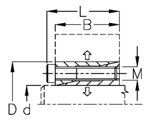
$\begin{array}{lll} \text{B mm} & = 21 \\ \text{d mm} & = 18.00 \\ \text{D mm} & = 35 \\ \text{Fit tolerance} & = \text{Aksel h8, Nav H8} \\ \text{F kN torque} & = 8.0 \\ \text{L mm} & = 25.0 \\ \text{M mm} & = M4 \\ \text{P N/mm2 surface pressure on shaft/hub} = 60 \end{array}$
